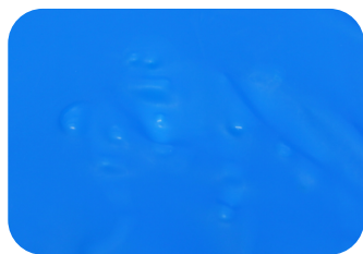
The latex dam shows localized distortion when contacted with chloroform which persists for over 10 minutes.
