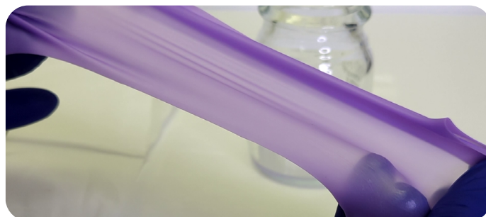
Polyisoprene True Dental Dam after 1 hour immersion survives stretching.
