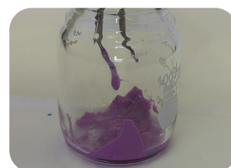
Flexi Dam after one hour immersion dissolved into a formless gel.
